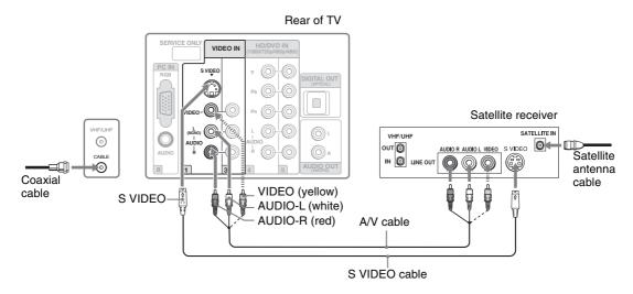
If your satellite receiver is not equipped with S VIDEO, use a VIDEO cable (yellow) instead of the S VIDEO cable.
