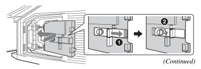
9 Put the outside lamp cover back in its place. Replace the cover, inserting it from the left side. Press the two tabs on the right side to secure the cover.
