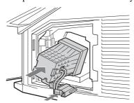
The lamp compartment is tilted, as shown in the following illustration.
